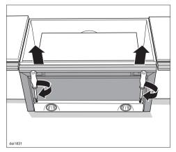
The position of the deflector plate can be brought forward by up to 35 mm using the adjusting screws on either side of the deflector plate.
